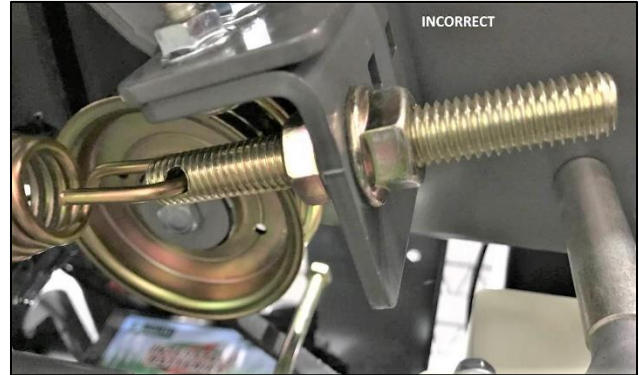
Figure 3: Incorrect Tensioner Adjustment
